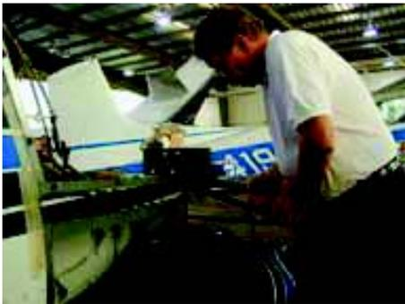
And the top strip is riveted back in with a doubler beneath it for the top fasteners.
