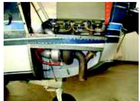
Here is what the STC does. The upper channel remains in place. Lower portion of cowling becomes removable.
